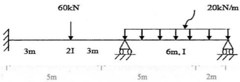
7. Analyse the continuous beam using flexibility method and draw the BMD and SFD
