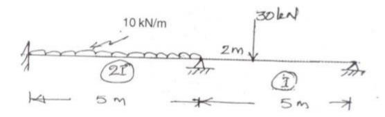
3. Analyse the continuous beam using stiffness method and draw the BMD and SFD
