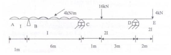
4. Analyse the frame using stiffness method and draw the BMD
