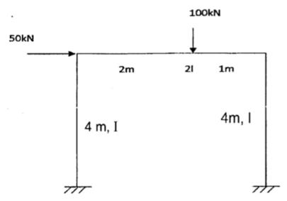
2. Analyse the continuous beam using stiffness method and draw the BMD and SFD
