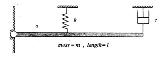
5. A mass m is suspended on a massless beam of uniform bending stiffness EI as shown. Derive the differential equation of motin for the system.
