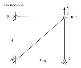
10. Derive the stiffness matrix for the structure with coordinates as shown in figure.
