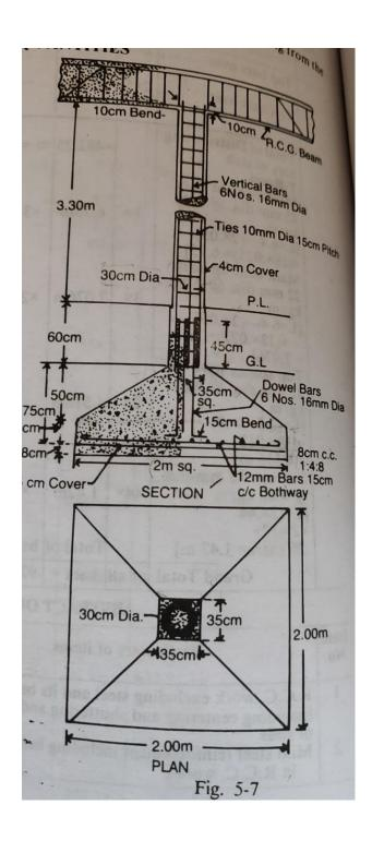
7. Prepare the detailed estimate of RCC retaining wallof 30m span from the given figure. Also prepare bar bending schedule 20 marks
