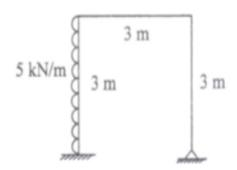
4. Analyse the frame using direct stiffness method and draw the BMD
